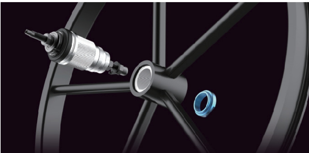
▲ The press-fit ratchet ring is used for better durability.
